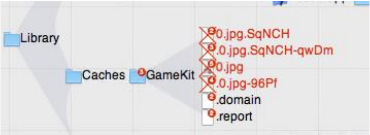
Figure 5. List of initial dropped files using a file event monitor tool
