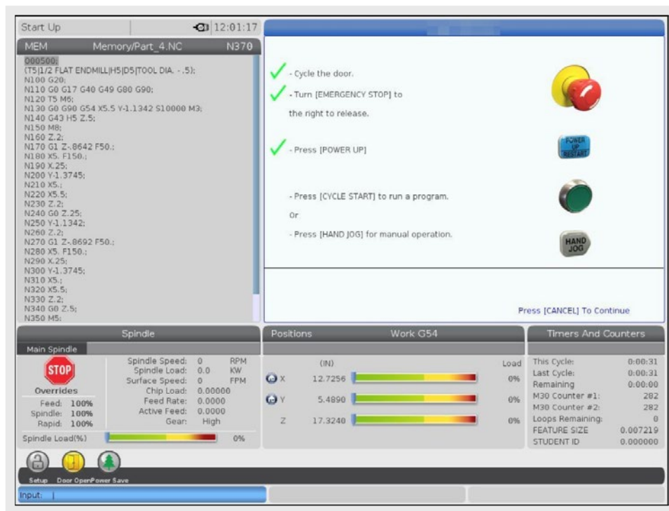
Figure 16. Menu showing instructions and readings for spindles and duration of cycles
