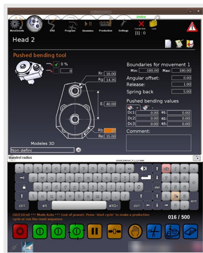
Figure 15. Exposed HMI for a bending tool
