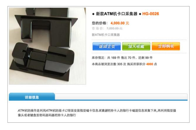
Figure 13: ATM skimmers cost RMB 4,000 (~US\$631) each; these came installed with a microchip that records payment card track data or the confidential information stored on a card's magnetic strip, along with a microcamera that allows cybercriminals to obtain a victim's PIN
