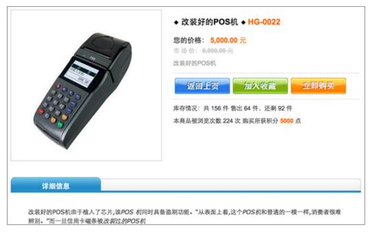
Figure 9: PoS skimmers are sold for RMB 5,000 (~US\$788) each on Izise.com; the site is run by a cybercriminal who specializes in selling customized PoS terminals that look no different from those that have not been tampered with, but come with a special chip that allows criminals to authorize otherwise unauthorized purchases
